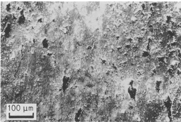
Figure 10 Example of a worn Y-TZP surface after a test against composite A9 at 8 N and 4 Hz for 24 h. The dark pits are identified as sialon fragments. This picture was taken with scanning electron microscopy at a magnification of 120\times .
